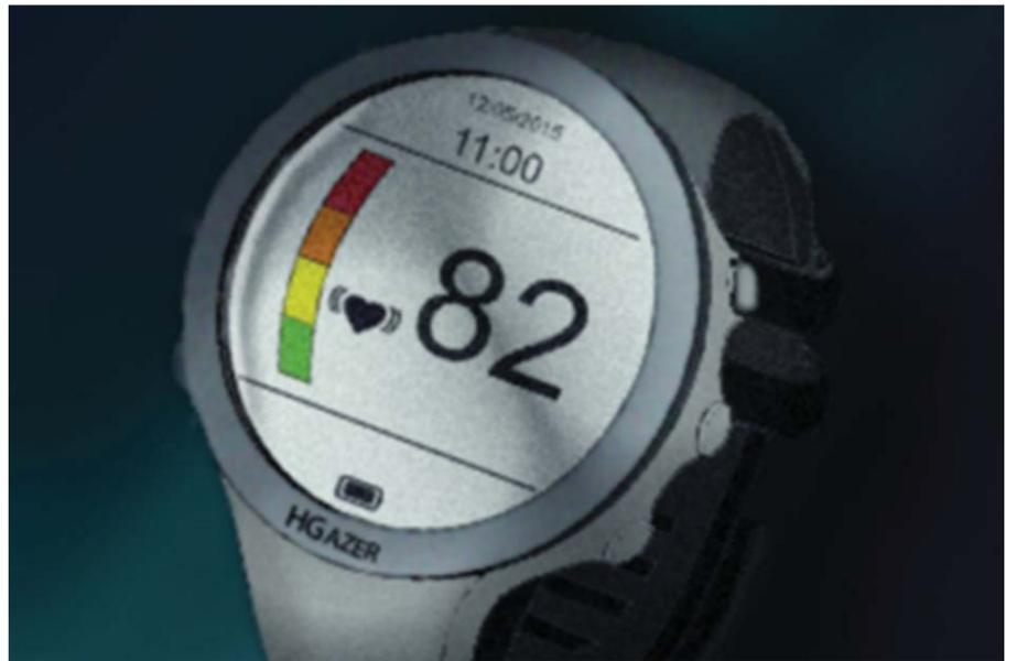
PS25251 EPIC UHI ECG Sensor. The developers have renounced electric motor-air pump into an air bag-cuff as well as the bag itself which make carpal tonometers inconvenient in everyday wear and consuming too much battery charge.
