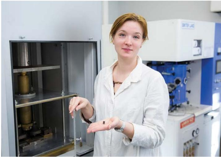
on electropower impact of powerful short-term (less than 1 msec) high-voltage electropulse and at the same time mechanical pressure on powder material. Material in the influence zone is warmed up to very high temperatures up to plasma condition. Pressure in the influence zone forms required properties of received products. The advantages of this technology are ecological cleanness, high efficiency: its energy consumption is 10 times lower than in the same
